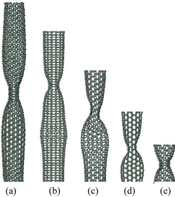
Figure 2. Buckled shapes for (7, 7) SWCNTs obtained from MDS.
